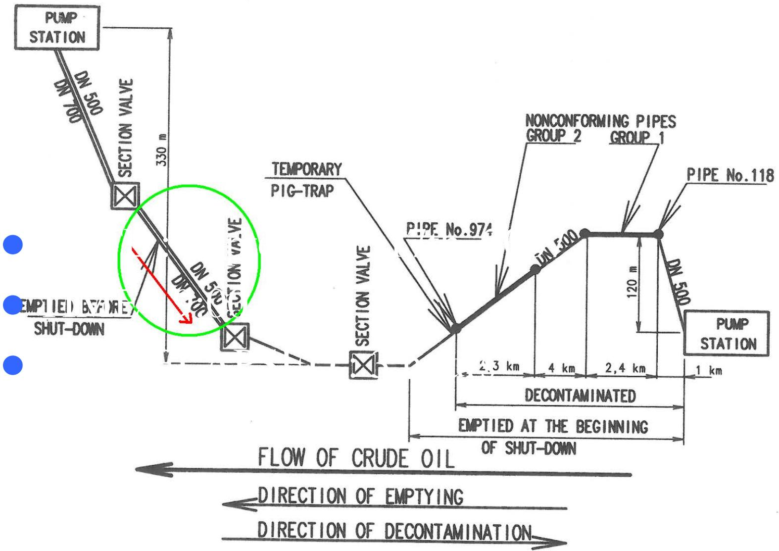
The last downstream pipe (No. 974), which was planned to be replaced, had been cut out using flameless technology. The next downstream pipe (No. 975) is closed by PLP sealing pig.
