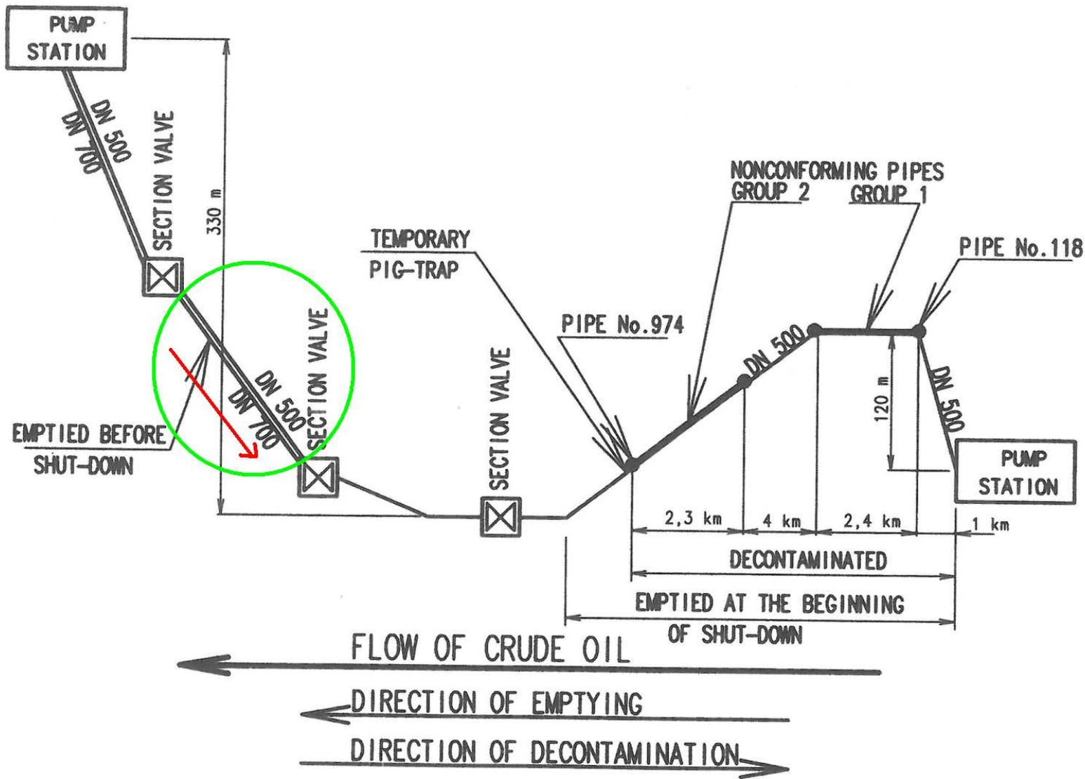
The crude oil was displaced to tank trucks at the lower end, and the oil was transported to storage site.
